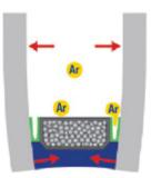
ProSeal remains gas-tight during unit expansion and compression cycles. Stress is evenly distributed across the spacer width, enhancing the retention of argon and energy efficiency.
